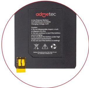
1. Begin by removing the protective foil from the battery terminals.
