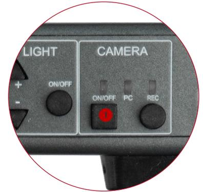
Turn off the camera by holding the **ON/OFF** button for three seconds.
