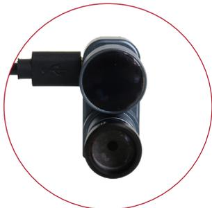
4. Connect the opposite end of the camera cable, the micro-USB connector, to the camera module.
