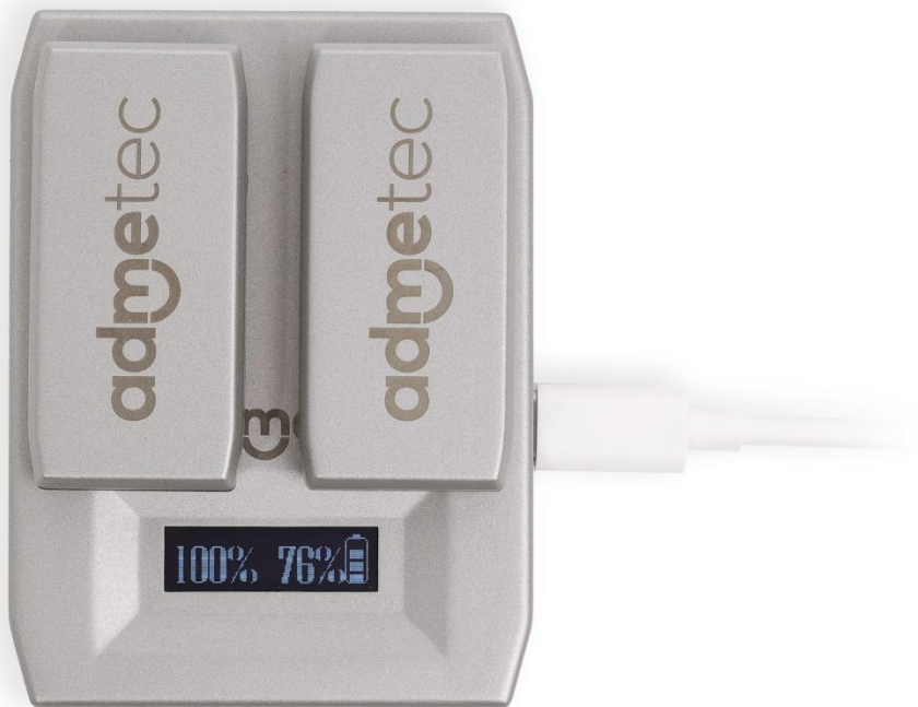
Fig. 02 – Batteries connected to charging pad.
