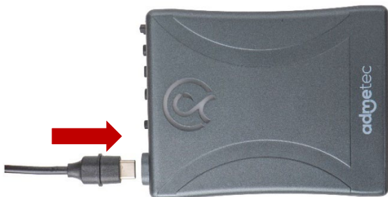
Fig. 03 – Type C cable insert into MCU
