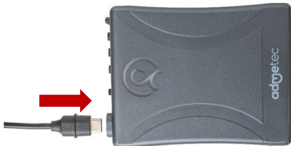
Fig. 03 – Type C cable insert into MCU
